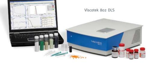
The patented single-mode fiber technology which lies at the heart of the unique optical system makes the 802 DLS far superior to all other DLS instruments.
