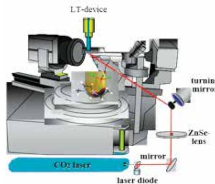
Apparatus for crystallizing ILs in situ on an X-ray diffractometer
