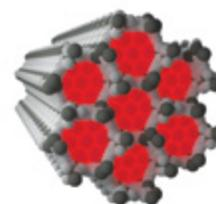
Neon observed experimentally within the pores of NiMOF-74 at 100 K and 100 bar of neon gas pressure. Figure courtesy of CCDC.
