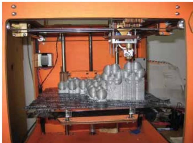
The extrusion printer has trouble starting the print at the bottom of an atom (sphere), so a software assist (in program CURA, which converts a .stl file to a .gcode file for my Ultimaker printer) builds a scaffold under nascent atoms. An 18 x 14 x 8 cm<sup>3</sup> model of Tasigna (PDBID 3CS9) with 1.5 x atomic radii is shown above.
