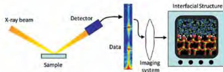
**Figure 1:** A highly idealized imaging system based on interfacial x-ray scattering: the x-ray beam is reflected from the surface of the sample (left), and the data are in the form of a "crystal truncation rod" (middle). What is needed is an imaging system (e.g., a lens or algorithm) that can create an image of the interface on the display (right) directly from the measured data.
