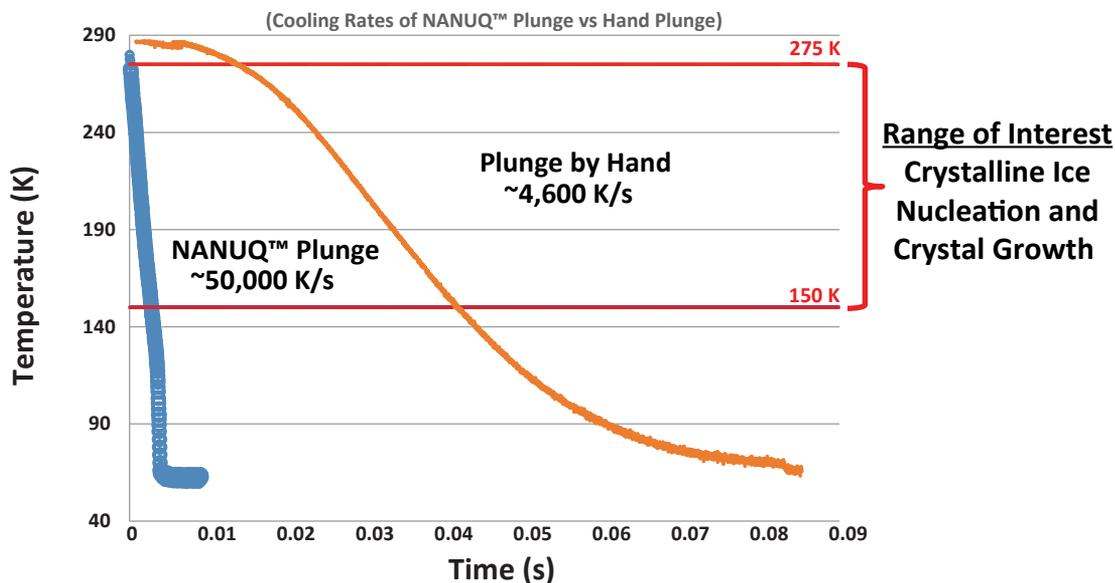
Hand-plunged crystals experience the majority of their cooling in the cold gas layer above the surface of liquid nitrogen (LN<sub>2</sub>). This produces a slow cooling rate that allows significant time for the nucleation and growth of crystalline ice.
