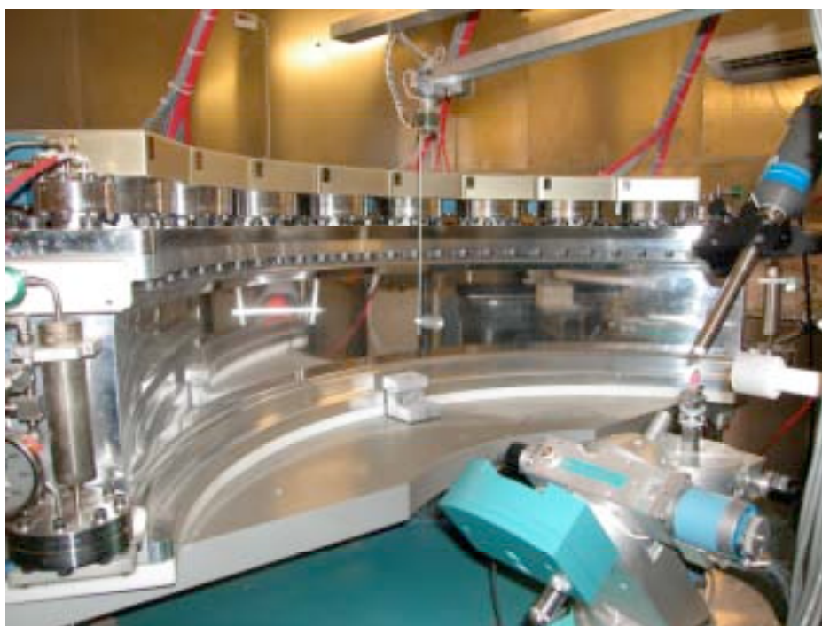
Figure 19. The large position sensitive detector built by the Instrumentation Division at BNL for the protein crystallography station at LANSCE.
